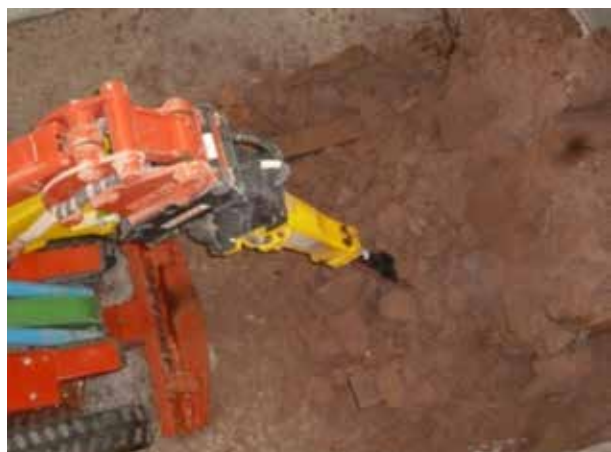
A converted digger is able to work with tools like angle grinders as well as to use the chipping hammer.
