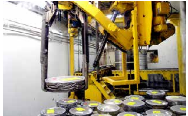
Incombustible components are compacted to pellets by high pressure.
