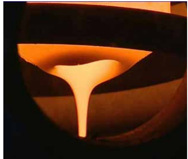
Filling glass from the melter into the canister.
