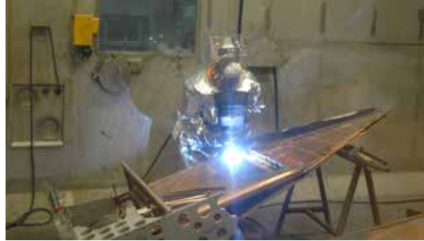
Large components are fragmented first and then decontaminated.
