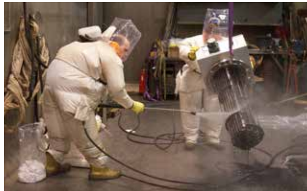
Decontamination by pressure water jet.
